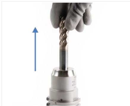
2. Remove the tool from the location bore of the HTC clamping chuck.
