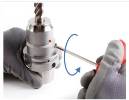
Fig. 12: Loosening clamping screw
