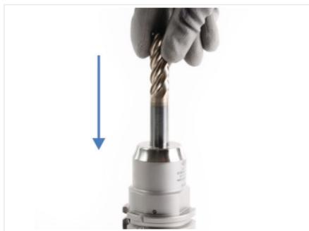
2. Push the tool, shank first, to the stop screw in the location bore in the HTC clamping chuck.
